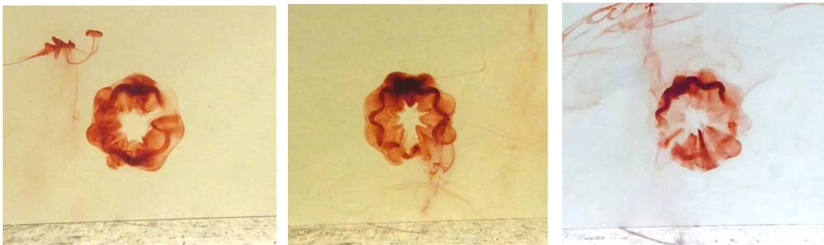
Figure 40 - Instability formed with various modes. A) 7 B) 8 C) 9
