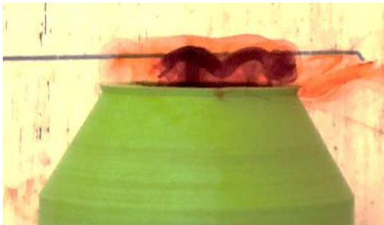
Figure 42 – 1 st iteration nozzle - shape production
